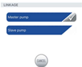
Fig. 20: In this menu, it can be determined whether a pump works as master or slave. Only one pump can work in master mode. Several "MASTER" pumps in the same area lead to unwanted interactions.
