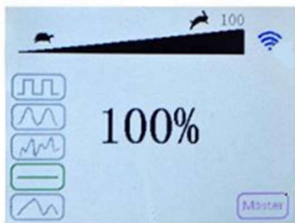
Fig. 2: Weergave pump controller
