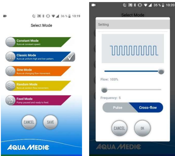
Fig. 26: ... then you tap on the wave symbol in front of "Classic Mode" and select "Cross-flow" (is then highlighted in blue). The pump power is adjusted under "Flow", the switch-on and switch-off time with "Frequency" (minimum approx. 30 seconds, maximum approx. 90 minutes). Save with "OK" and "Save". It can take up to three cycles for the pumps to "find" their alternation rhythm. You should therefore start with a cycle at the lowest level and increase it when the pumps change evenly.
